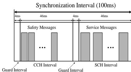
Fig. 1: The multichannel MAC scheme used by DSRC
