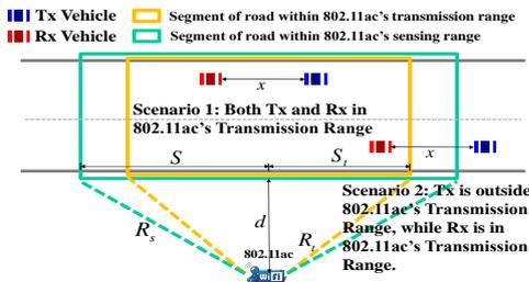
Fig. 2: Locations of the DSRC nodes and the 802.11ac node.
