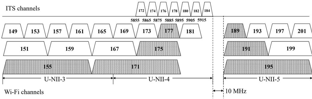
Fig. 2: ITS channels and U-NII Wi-Fi channels. The shaded channels indicate those adjacent channels that can interfere with ongoing C-V2X operations.
