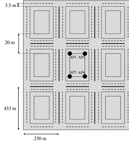
Fig. 3: The Manhattan grid layout and location of Wi-Fi APs
