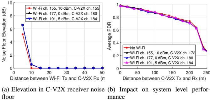
Fig. 9: Impact of Wi-Fi power on C-V2X performance
