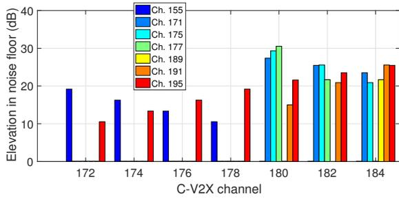
Fig. 6: Elevation in the noise floor for C-V2X receiver
