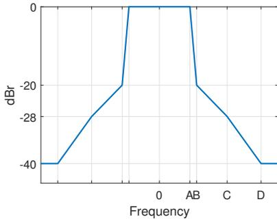
Fig. 1: The default (class A) spectral mask for Wi-Fi
