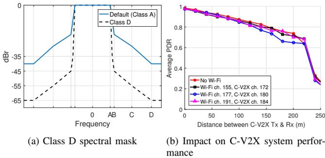
Fig. 8: Impact of Class D mask on C-V2X performance
