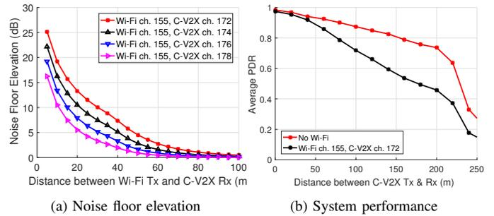
Fig. 5: Impact of U-NII-3 adjacent channel interference on C-V2X performance
