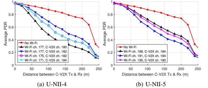
Fig. 7: Impact of U-NII-4 and U-NII-5 adjacent channel interference on C-V2X performance
