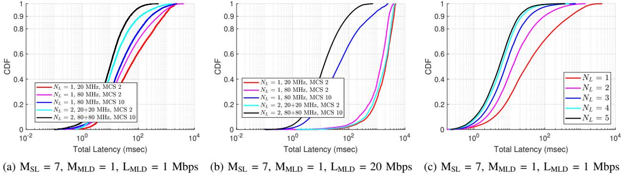
Fig. 4: CDF of the end-to-end latency of the MLD's packets. One MLD competing for channel access with single-link STAs.
