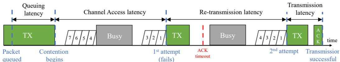
Fig. 1: Illustration of latency components in Wi-Fi;  $(CW_{\min}, BO) = (16, 7)$  for attempt 1, and  $(32, 4)$  for attempt 2.
