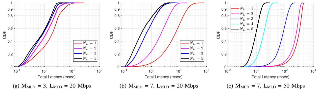
Fig. 5: Impact of traffic prioritization and multiple MLDs on the MLDs' end-to-end latency,  $M_{SL} = 7$ .
